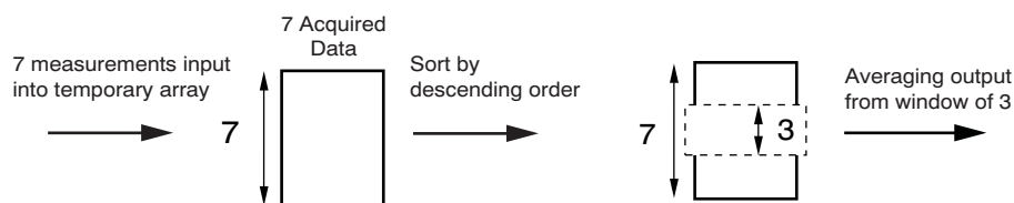
Figure 28. MAV Filter Operation (Patent Pending)
